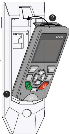
Figure 2-5 Installing the MDKE9 keypad into the base
